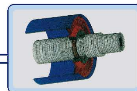
滚筒有限元分析 Finite element analysis of conveyor pulley
